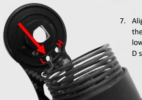
7. Align the OSPW front cage plate with the back of the derailleur, inserting the spring post into the low (L) tension setting on the cage. Aligning of the D shaped interface will be done later.
