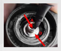
5. Mark the center screw end with a pen to identify the flat surface of the D on the bottom of the center screw (A).
