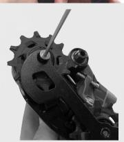
2. Remove the rear derailleur from the bike. Remove both pulley wheels and the back side of the pulley cage.
