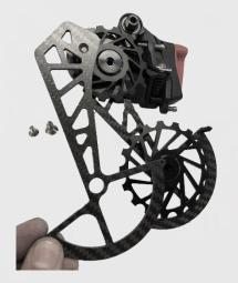
10. Install the 14T pulley wheel on the upper post and the 17T pulley wheel on the lower post of the OSPW cage. Align the back cage on the OSPW and tighten the silver screws on the backside.
