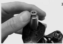
3. Hold the Sram pulley cage & derailleur, loosen the main center nut with the NOVA RIDE tool. Do not completely remove the mounting nut. When the center nut is loose enough, allow the rotation stop screw to move past the stop point on the derailleur body to release the spring tension.
