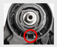
6. Mount the Sram spring back into the derailleur body. Be careful to place the spring post into the correct hole. Note: one hole is deeper than all others (see circle). Ensure the spring sits completely into the derailleur body all the way around.
