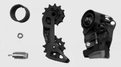
Remove the main center nut and the Sram cage. Set aside the spring and center nut for reuse.
