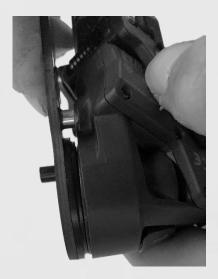
8. Mount the cage on the center screw and thread the center mounting nut into place using the provided 4 prong tool. Finger tighten the nut until firm, and then unthread 360 degrees (1 full turn). The D-interface will not be aligned at this point.
