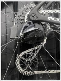
11. Install the derailleur on the bike. Shift down to the bottom (smallest sprocket) and install the rear wheel. Measure a new chain and check the upper and lower stop screws as well. Add the b-limit adjustment following the SRAM guidelines: 14mm for a 26T sprocket, 10mm for a 28t sprocket, 5mm for a 33T sprocket.
